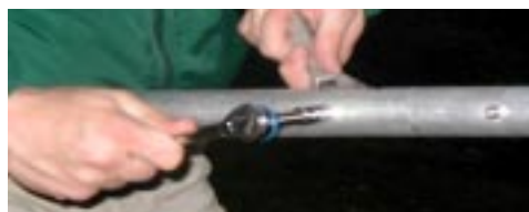
Figure 4: Securing the boom sections
