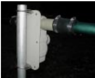
Figure E: Mounting the dipole to the mast
