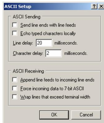
Figure 5. ASCII setup window. It's critical that these Parameters are set exactly like shown
