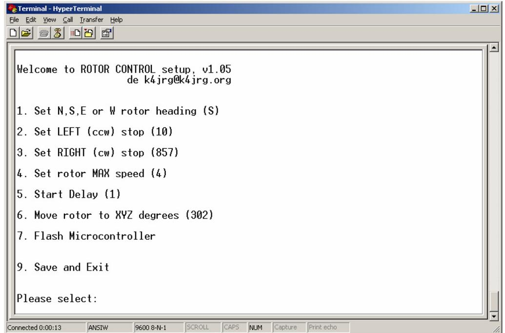
Figure 1. User Interface Main Menu. Activated with the **UI** command
